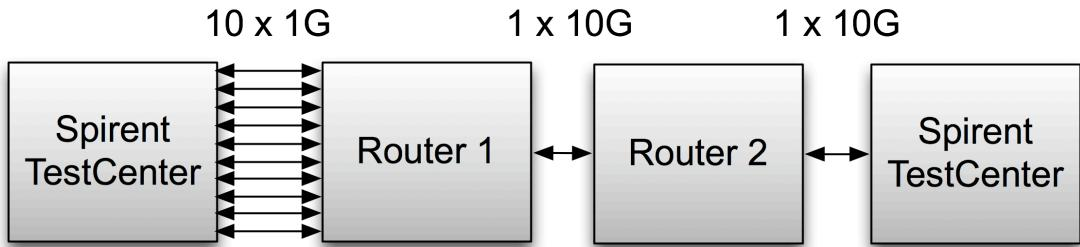
In the figure above, Router 1 on the left-hand side of the diagram represents a data-center device terminating many IPSec tunnels, while Router 2 on the right-hand side of the diagram represents multiple routers at remote sites.
