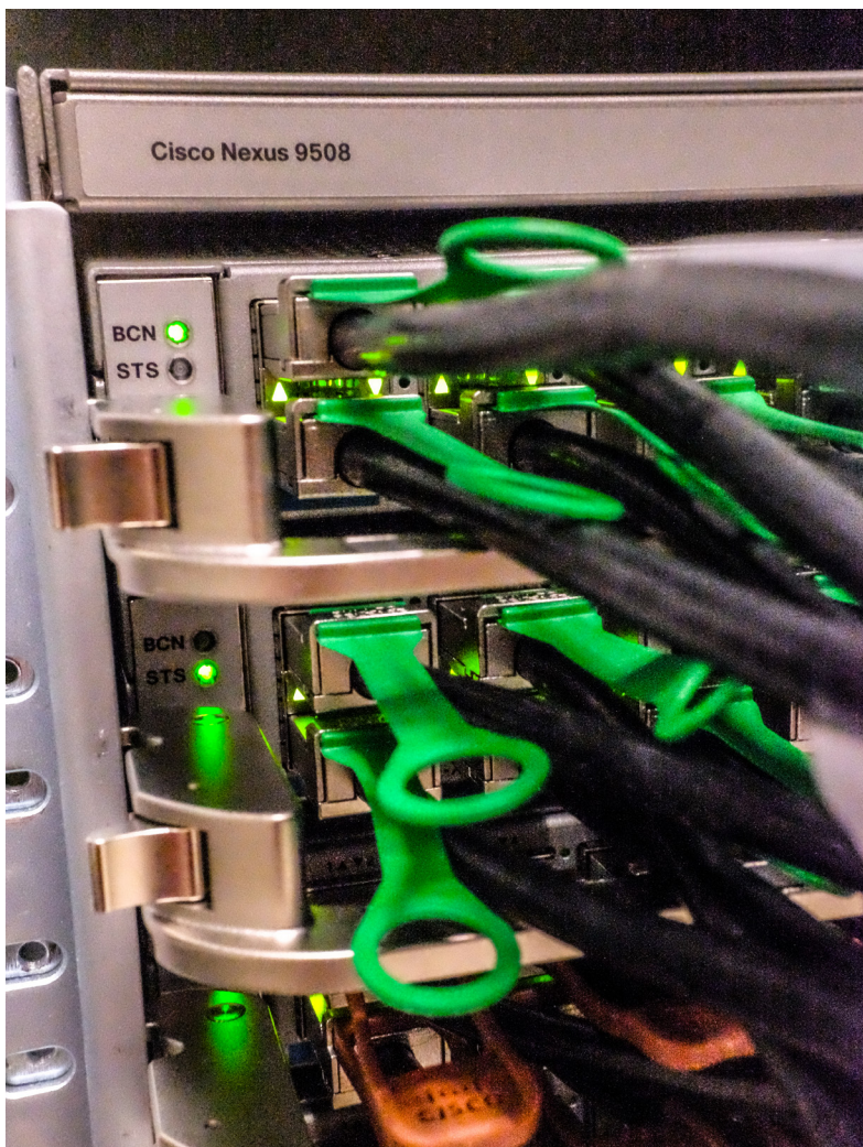
Figure 1: The Cisco Nexus 9508 on the test bed with 256 100G Ethernet ports
