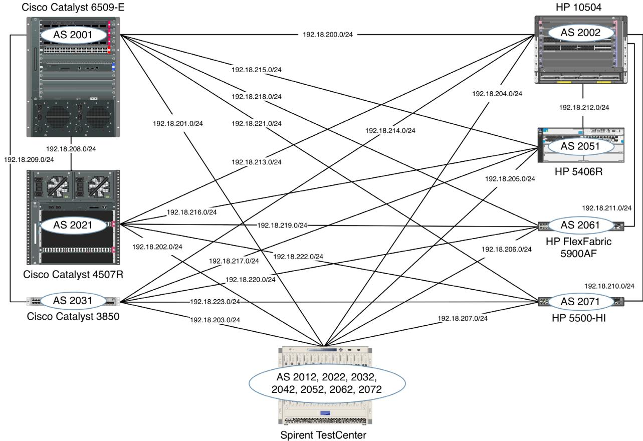
Figure 2: BGP interoperability test bed
