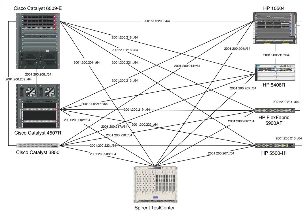
Figure 7: OSPFv3 test bed
