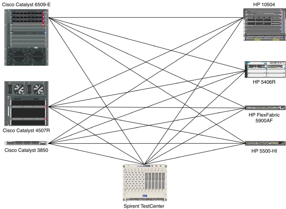
Figure 8: Spanning tree protocol test bed
