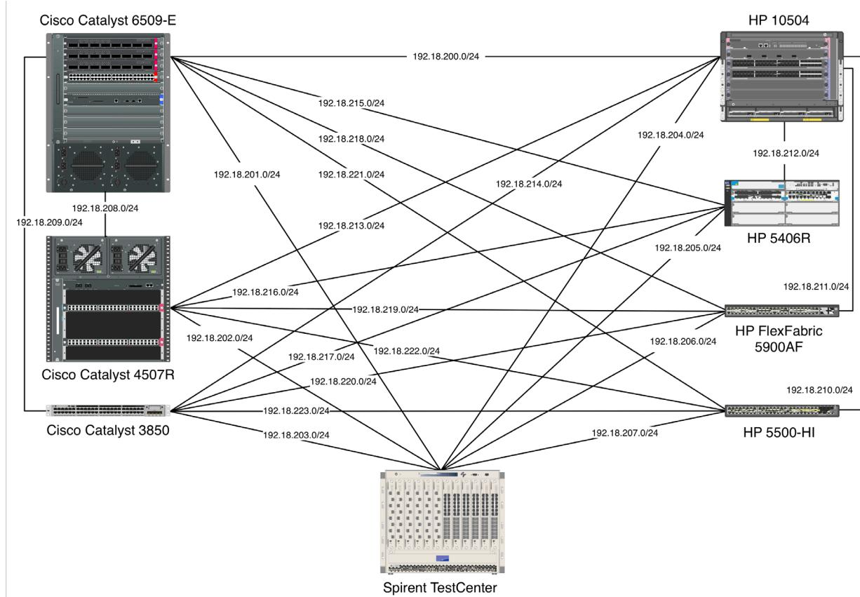
Figure 6: OSPFv2 test bed
