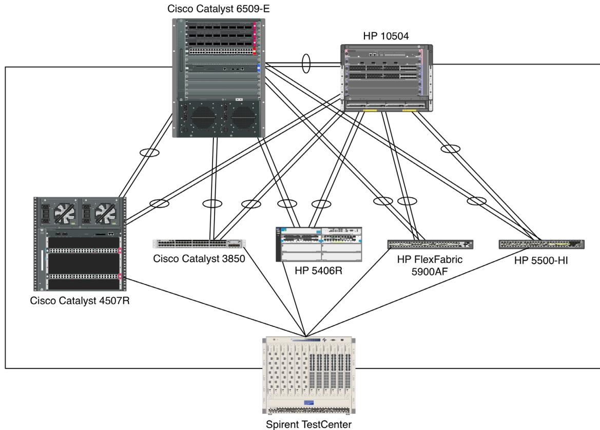
Figure 5: Link aggregation test bed
