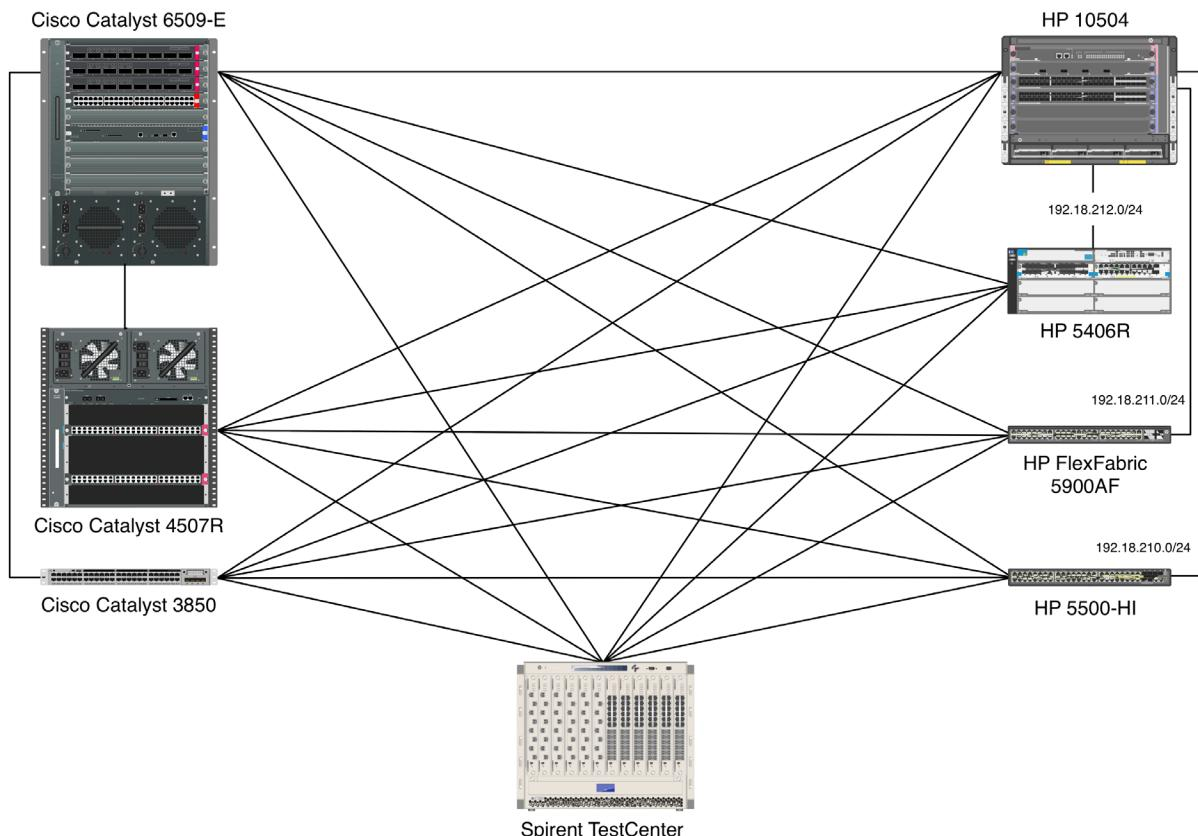
Figure 3: The CDP interoperability test bed
